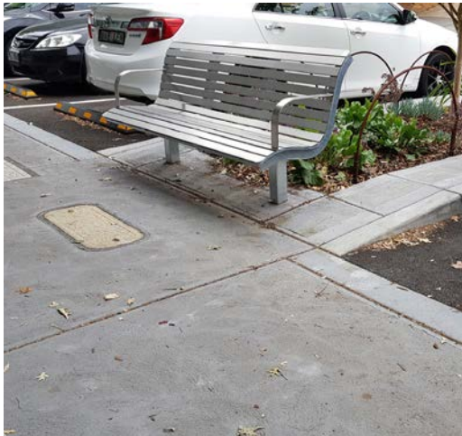
Type: Council standard bench seat Dimensions: 1800L x 685W x 870H Materials: Mild steel & stainless steel
