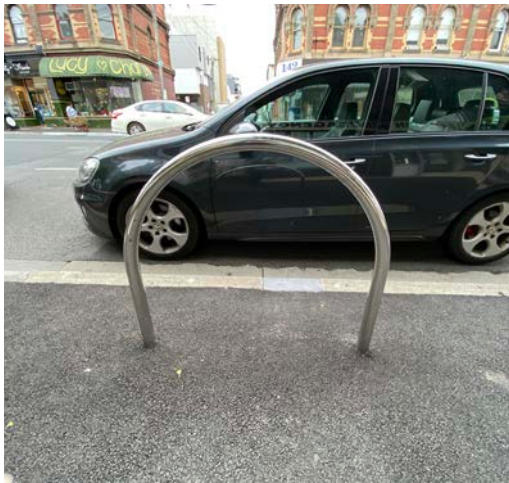
Type: Council standard bike rack Dimensions: 1000L x 900H Material: Stainless steel
